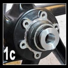
2) Next, we'll fit the fork bush (TYLY-0121B) which is used to reduce the diameter of the bore to match up with the new axle shaft.
