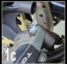
2) Use the bolts provided to secure the calipers to the mounts
