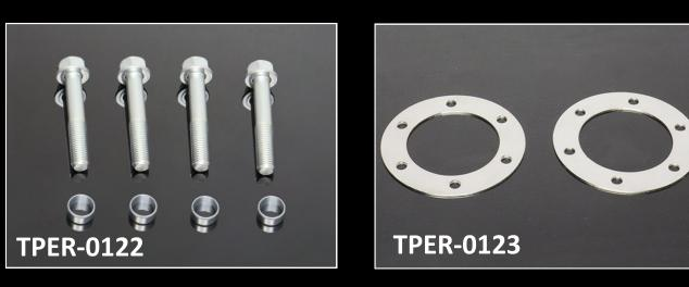
This CBR1000RR 2008-13\* fork conversion kit is designed to allow the CBR1000RR front forks to be used on your NC30/35, MC21/28, MC22 etc. and used the OEM front wheel from your original bike, or a number of Honda front wheels from the late 80's early 90's.
