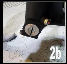
**3)** When the time comes to fit the wheel to the fork, note that the axle shaft is inserted from the right side and should be pushed all the way in until the right hand end of the shaft is flush with the outer face of the right hand fork leg. Use the axle bolt from your original bike to secure. In our case the bolt is MC21/28.
