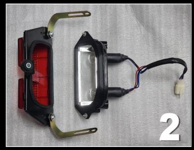
3) The bulbs (12V-18W/5W) are bayonet type, so just pop out the old and fit the new.
