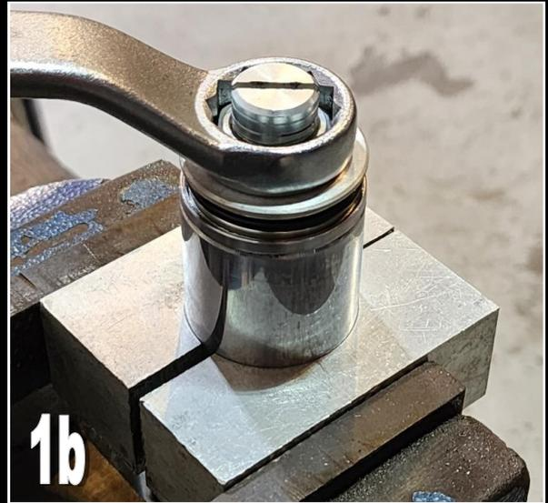
2) Now clamp the forks in the vice vertically and undo the caps completely from the fork tube.
