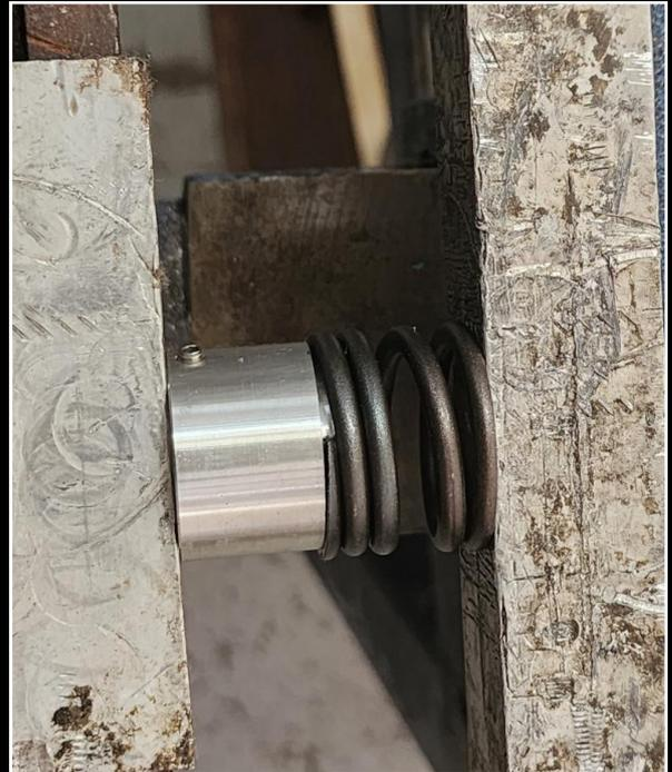
**12)** Now fit this assembly onto the cartridge. Make sure that it is fully seated and tighten the grub screw. We advise using some Loctite 263 high strength threadlocker compound on the grub screw so that it cannot come loose.
