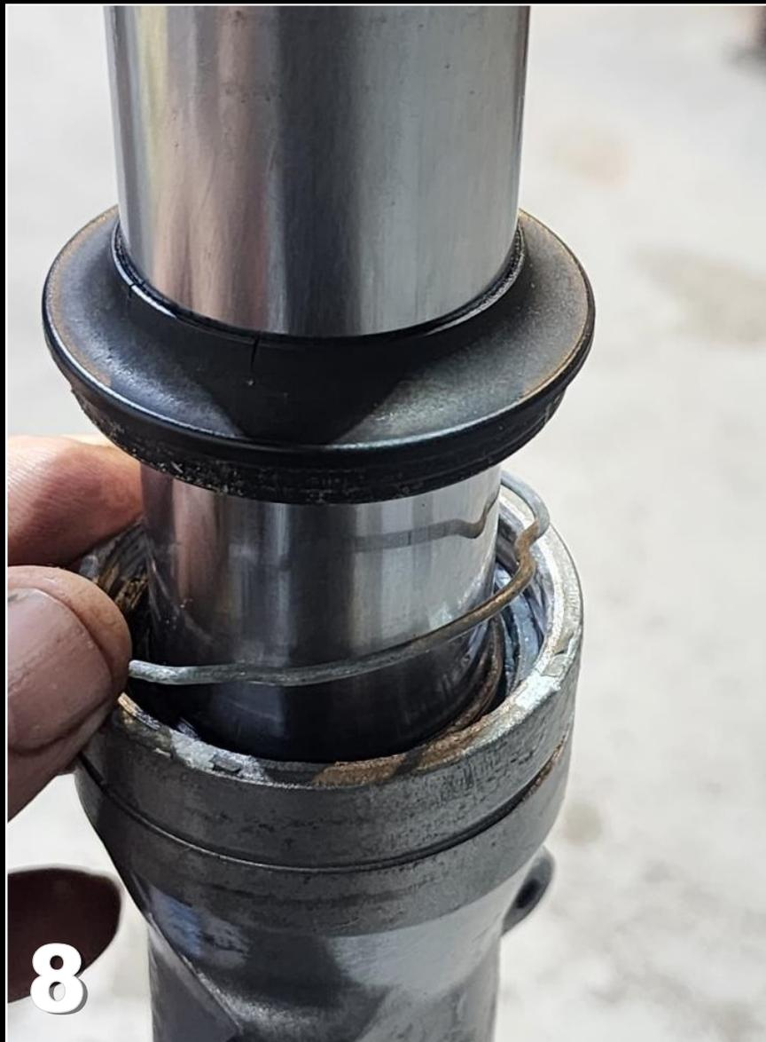
And now we must get a bit aggressive to remove the seal, back up ring and fork bushing. Lock the fork lower in the vice with soft jaws, and use the inner tube as a slide hammer, pulling it abruptly to full extension. This will remove the seal, back up ring and bushing.
