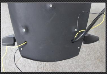
11) The next job is to secure the exhaust stay to the undertray. This is actually a bit of a fiddly job due the rubber bushes. First assemble the rubber bushes (as shown in the images below) on the legs of the stay. Then insert the legs of the stay through the undertray and work the rubber bushes into
