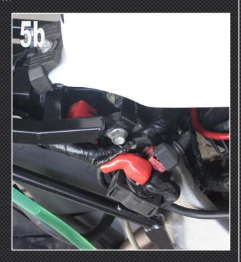
6. The coil is mounted on the lugs near the tank position. Use the original bolts. Connect the coil to the main harness later once the harness is in position.
