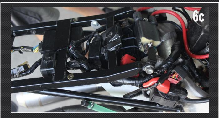
7) The regulator/rectifier is mounted on left of the subframe. Note that the NC30 and NC35 have different pitch hole positions so there are 3 holes provided. If the regulator/rectifier has an aluminium heatsink, we recommend reinstalling it between subframe and R/R. We provide mounting Connect the regulator/rectifier to the main harness later once the harness is in position
