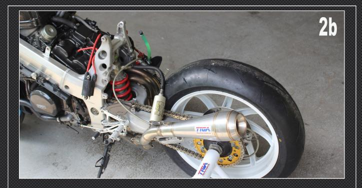
**3)** Fitment of the Tyga subframe is next. This is secured the same way as the stock one but this time use the two special bolts BPSY-0049 supplied in the subrame kit for the lower mounts. These have M4 threads in the heads of the bolts used for securing the bodywork later. There is some adjustment in this component, so make sure it is exactly center and perpendicular to the bike before tightening the bolts to 40 Nm.
