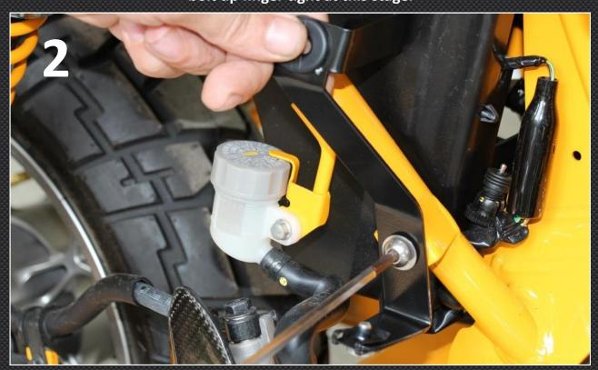
3) Secure the stay to the plastic 'luggage box' using the M6 screw, washers and M6 nylok nut. Again, just finger tight.
