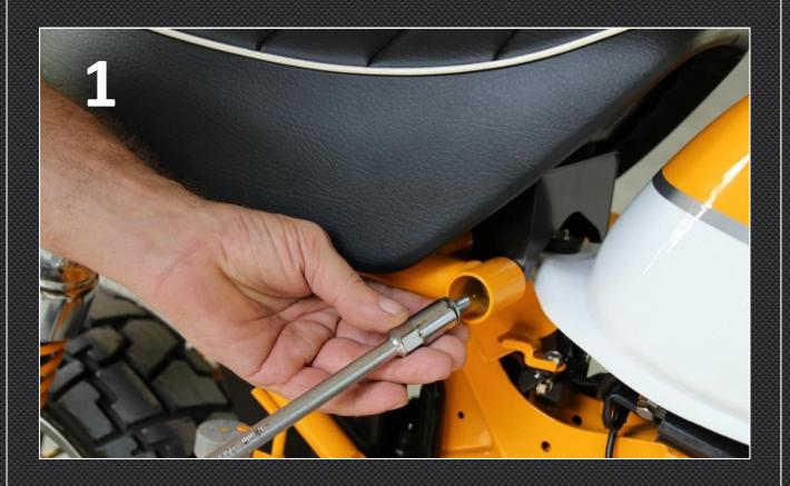
2) Secure the stay BPSY-0231A to the frame using the M8 button head bolt. Just nip the bolt up finger tight at this stage.
