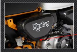
Press on the R. Cover by pushing the spigots into the rubber grommets, and tighten the M6 screw on the underside securely.
