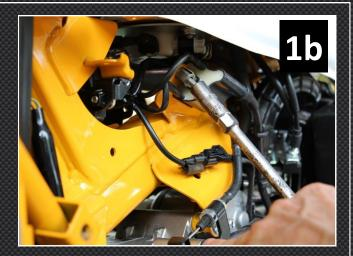
2) The stay BPSY-0231B is located atop the coil and is secured with the 2x M6 cap head bolts and washers provided.
