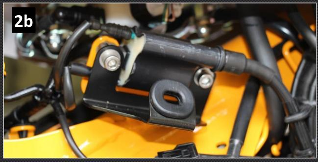
Now offer up the R. Cover (BPCC-7142R) and check that the **spigots** line up with the rubber grommets, and that the M6 clip on the underside lines up with the **hole** in the R. Cover.
